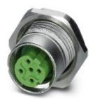
Bus system flush-type socket, with green contact carrier, 4-pos., M12 SPEEDCON, shielded, D-coded, rear/screw mounting with M16 thread, with straight solder connection
