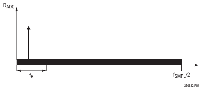
Figure 15. Frequency Spectrum of SAR ADC Core Output
