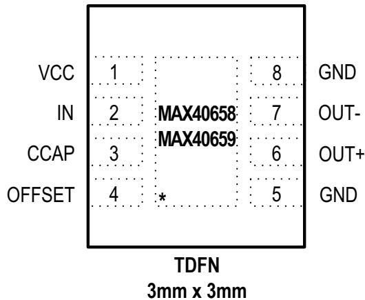
\*THE EXPOSED PAD MUST BE CONNECTED TO THE CIRCUIT BOARD GROUND FOR PROPER THERMAL AND ELECTRICAL PERFORMANCE.
